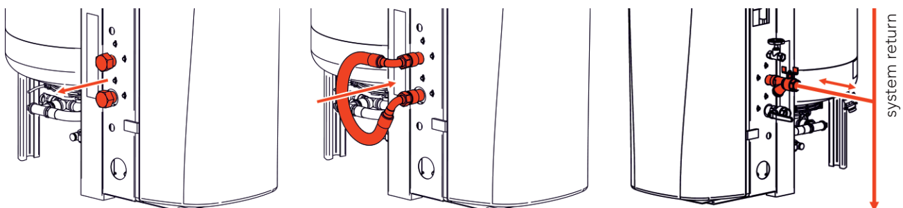
figure 6: connection via multicontrol kompakt bypass set and connection to the system return
