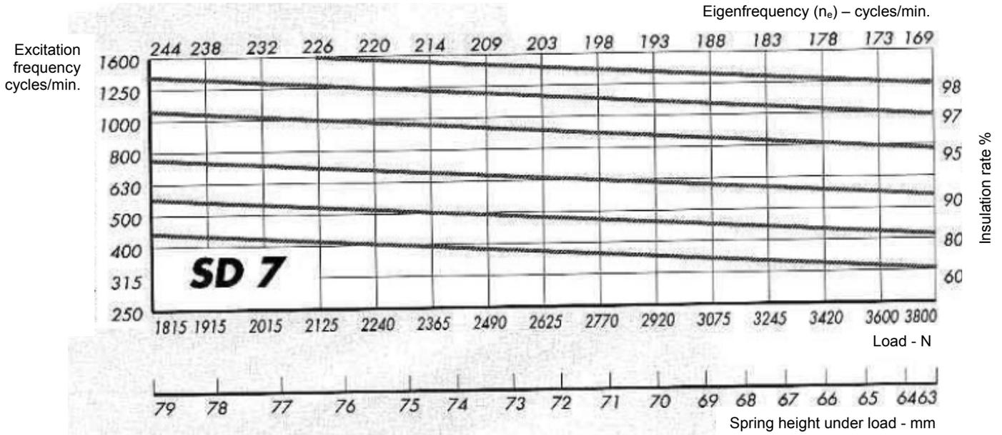
The ratings of the spring anti-vibration devices featured on the LCX Frame 6 units are show in the diagram below:
