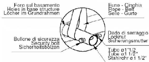
Use ropes or belts long enough to extend beyond the height of the unit and place spacer bars and boards on the top of the unit to avoid damaging the sides and top of the unit itself. The rectangular holes are provided for the attachment of vibration damping supports (optional).
