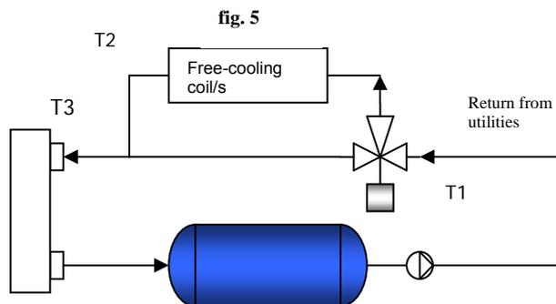
The 3-way valve can also be placed manually in the event of faults occurring in the actuating booster: the figure below illustrates the position of the 3-way valve...
