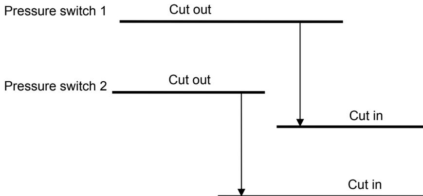
...where pressure switch 1 is set at the “PS” (maximum admissible pressure) of the system, while pressure switch 2 will have the setting = PS x 0.9 in accordance with the reference technical standard.
