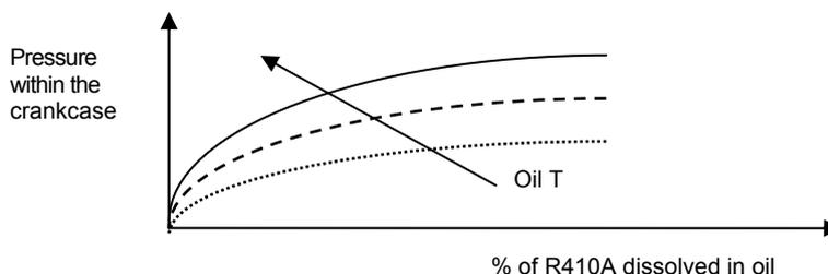
Use of electrical resistances is extremely important especially at the first start-up. It is recommended to leave them inserted for at least 12 hours before starting the compressors.
