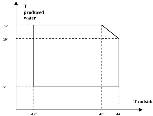
The lower limit is due to the limit of freezing temperature of glycol solutions with 35% of their weight made of glycol, the maximum admitted by the tightness of the pumps used.
