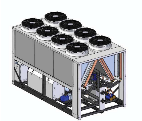
Free-Cooling unit in silenced FL version with 2 chilling circuits and 6 partialization steps. Detail of hydronic part on water connection side.
